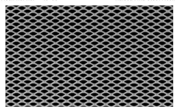
LW Pitch:10.00mmStrand Width:1.17mmSW Pitch:5.64mmThickness:0.9mmWeight:2.93 kg / m2Open Area:58%
